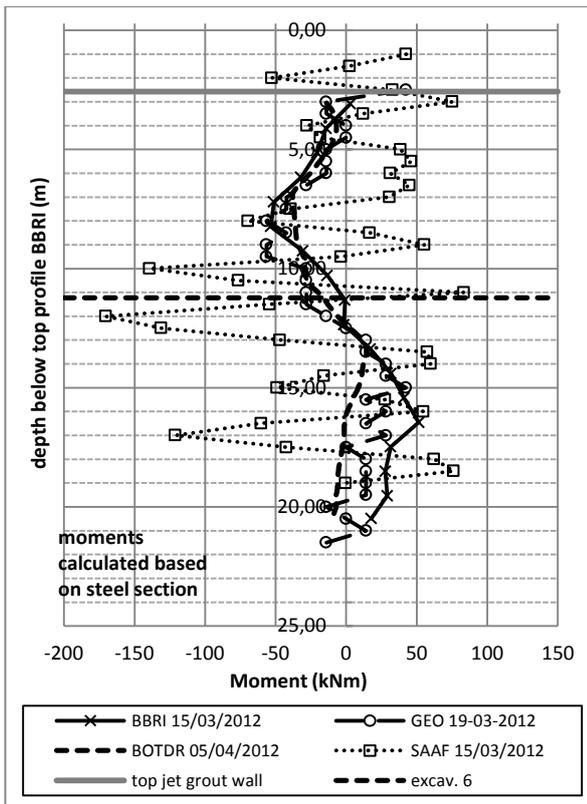
Figure 6. Bending moment HEB profile after the last excavation.
