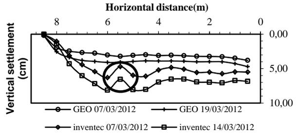
Figure 8. Settlements measured with hor. SAAF and hor. inclinometer.
